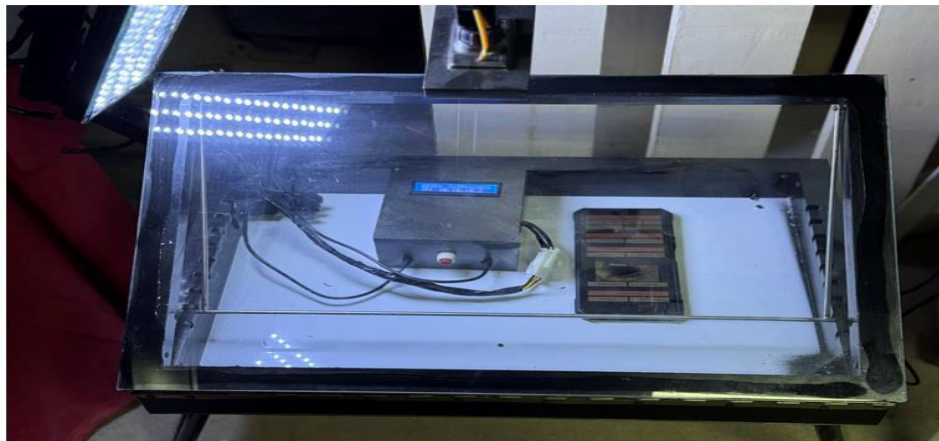
Figure 4. Technology Package (T-Pack) controller of the Portable Drawing Table
